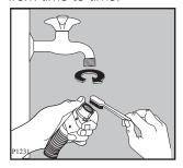
Turn off the water tap. Unscrew the water inlet hose. Clean the filter using a hard bristle brush. Refit the inlet hose.
